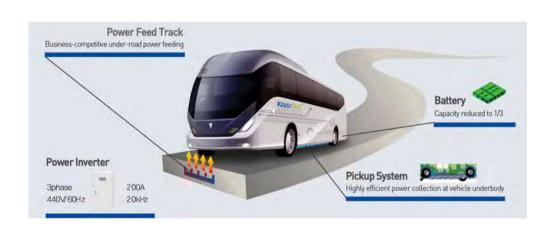
Solving battery and charging problems with OLEV technology, which enables wireless electric power transmission while vehicle is stopping or running.
